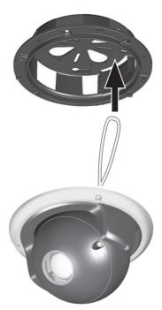
6. Suspend the camera module from the plastic hook inside the mounting base ensuring that the suspension cable is seated securely in the groove.
